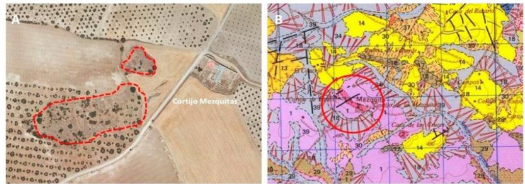
Figure 5. (A). Dolomite, limestones and carniola outcrops (Iberpix, IGN). (B). Geological map of the Cortijo de las Mezquitas area, with outcrops of variegated clays and sands in purple, and outcrops of dolomite and dolomitic breccias in red (Antequera Sheet 1023, IGME).
